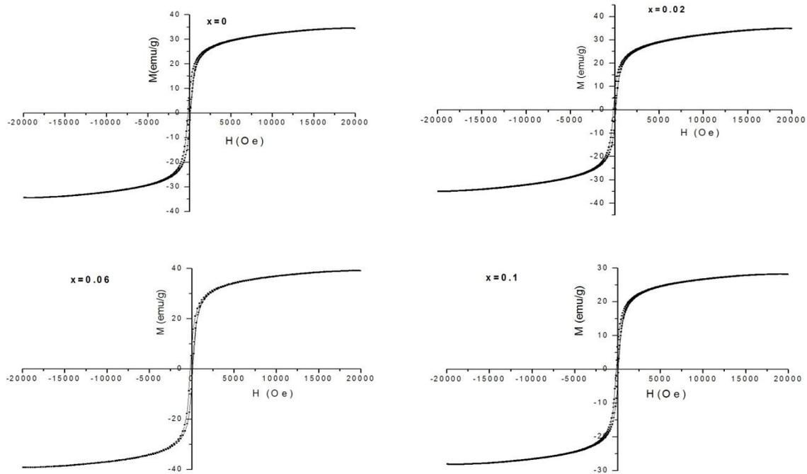
**Figure 4** Room temperature hysteresis loops of  $Ni_{0.9}Cd_{0.1}Tb_xFe_{2-x}O_4$  ferrites.
