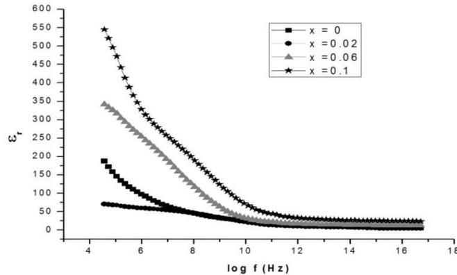
**Figure 6** Variation of dielectric constant with frequency for N-Cd-Tb ferrite system
