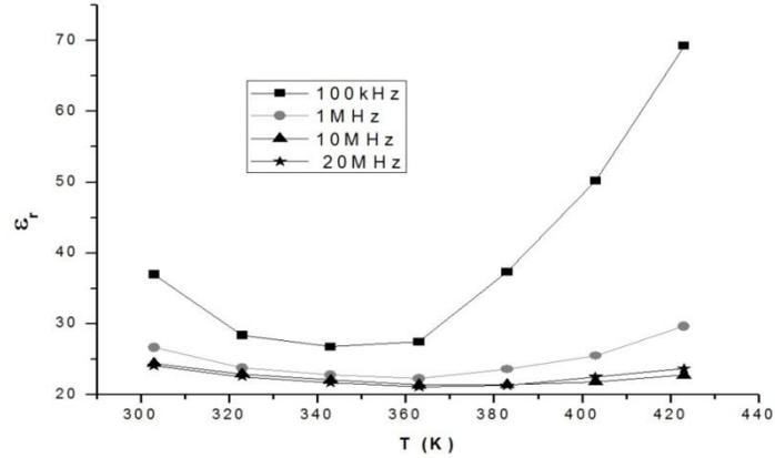
**Figure 7** Temperature variation of dielectric constant for the sample with  $x=0.1$  at selected frequencies
