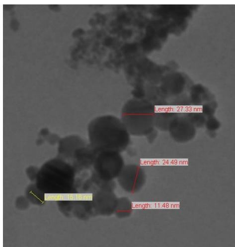
**Figure 2.** TEM image of  $\text{Ni}_{0.9}\text{Cd}_{0.1}\text{Tb}_{0.1}\text{Fe}_{1.9}\text{O}_4$  nanoparticles.
