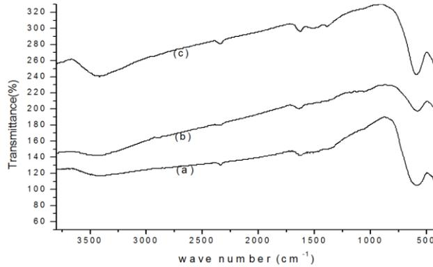
**Figure 3** Infrared spectra of  $\text{Ni}_{0.9}\text{Cd}_{0.1}\text{Tb}_x\text{Fe}_{2-x}\text{O}_4$  ferrites with (a)  $x=0.02$ , (b)  $x=0.06$  and (c)  $x=0.1$ .
