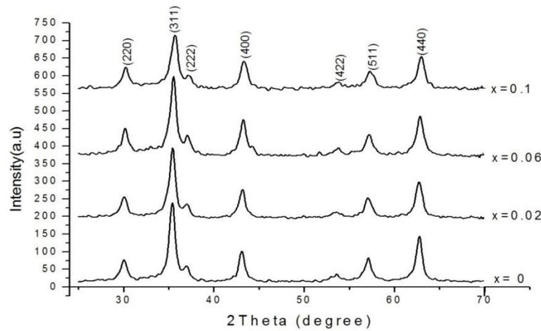
Figure 1. X-ray diffraction patterns of  $\text{Ni}_{0.9}\text{Cd}_{0.1}\text{Tb}_x\text{Fe}_{2-x}\text{O}_4$  ferrite system.
