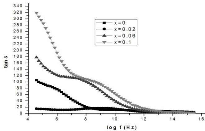
**Figure 8.** Variation of loss factor with frequency.
